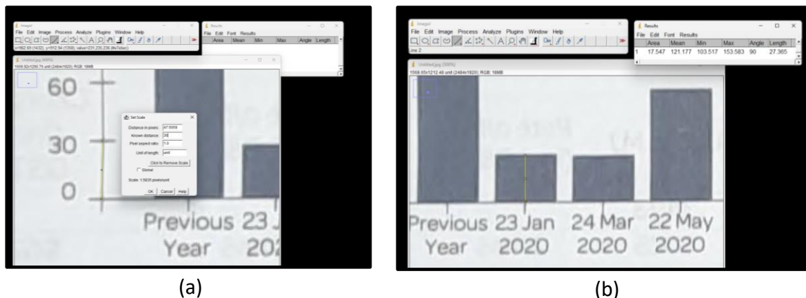
Figure 18. Calibration (a) and measuring values (b) of a bar graph from a gas bill using ImageJ software.
